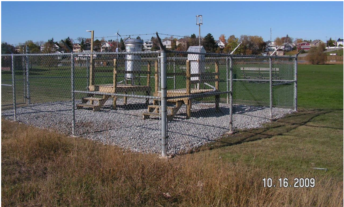
Figure 1: Photo of Air Sampling Station at the MRCA Office Site
